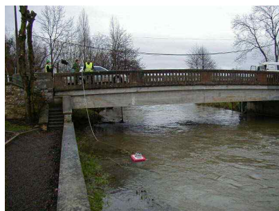
measurement at bridge (stationary measurement)
